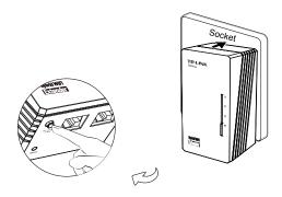
4. Place the extender in your desired location. The extender will automatically synchronize wireless settings with the router whenever the router's wireless settings are changed.
